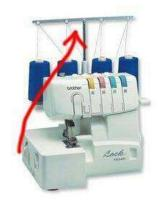
Make sure the thread are seated firmly in the thread channel by "flossing" the thread in the channel you will feel it when it seats properly and providing a little more resistance. Make sure the Thread Tree is extended all the way to full height.
